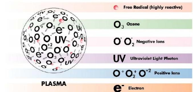
There are various ways to produce plasma, but the preferred method is the use of radio frequency excitation at 13.56 MHz. The highly energized non-equilibrium plasma is capable of surface cleaning and surface activation through physical, chemical, and physical/chemical mechanisms without changing the bulk properties of the materials. The degree of selectivity, anisotropy, uniformity and cleaning rates are a function of process parameter selection.
