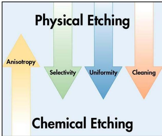
The process parameters also dictate whether the process is physical, chemical or a combination of these mechanisms. Each have distinct advantages and disadvantages when it comes to cleaning bond pad sites. The selection of the process gas, the chamber pressure, the power applied, and the time of the process determine the type of cleaning mechanism and its effects. These are the key process parameters.
